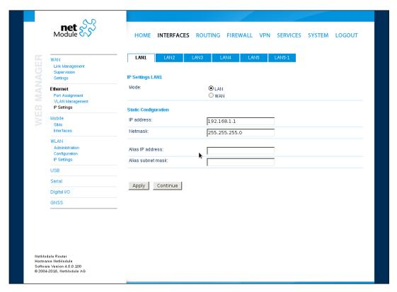
Figure 5.9.: LAN IP Configuration
