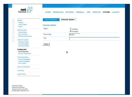
Figure 5.54.: Automatic File Configuration
