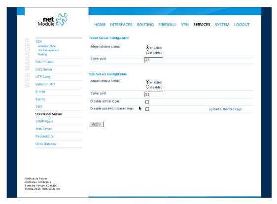
Figure 5.44.: SSH and Telnet Server
