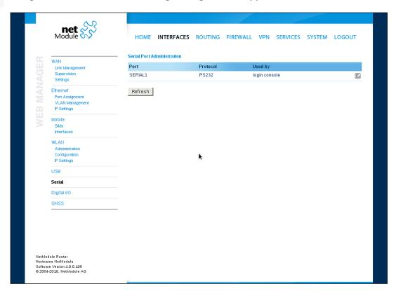
Figure 5.18.: Serial Port Settings
