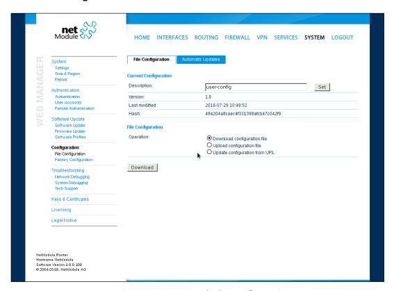
Figure 5.53.: Manual File Configuration
