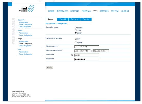
Figure 5.33.: PPTP Tunnel Configuration
