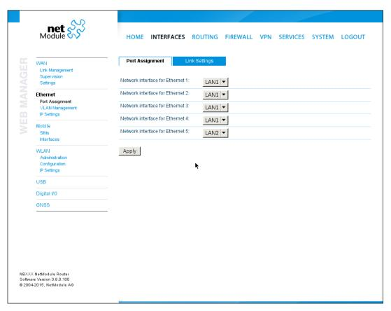
Figure 5.6.: Ethernet Ports
