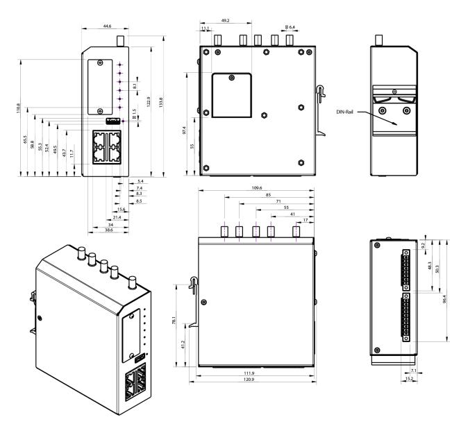
**Note:** Outline with A1-A5 antennas (2x LTE, 2x WLAN/BT, 1x GNSS). Order Number e.g. NB1601-LWWtSc-G (with COM/IO shield EXT 1, without extension EXT 2)
