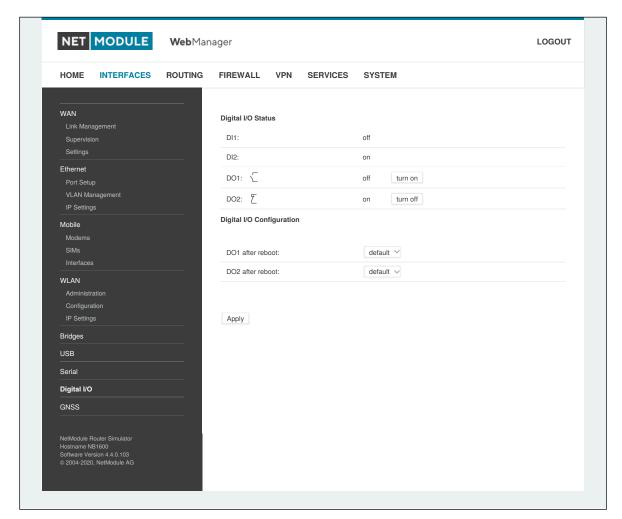
Figure 5.19.: Digital I/O Ports
