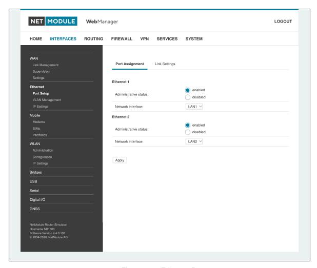
Figure 5.6.: Ethernet Ports
