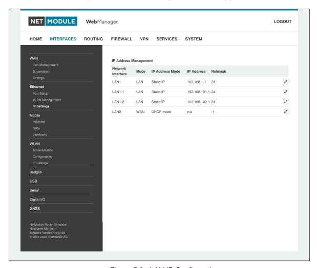
Figure 5.9.: LAN IP Configuration
