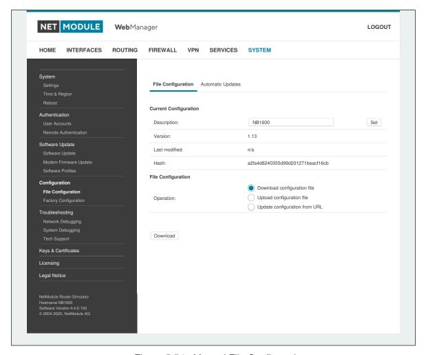
Figure 5.54.: Manual File Configuration
