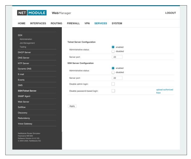
Figure 5.45.: SSH and Telnet Server
