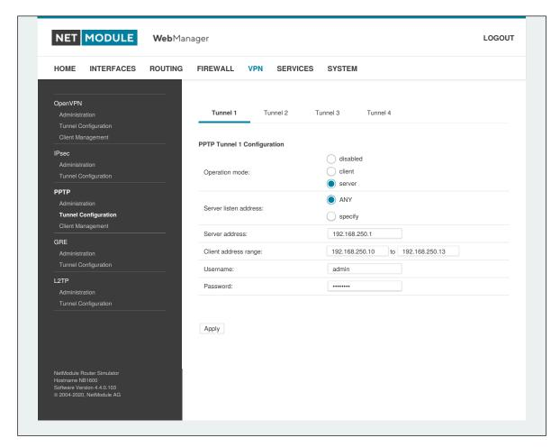
Figure 5.34.: PPTP Tunnel Configuration
