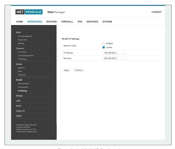
Figure 5.14.: WLAN IP Configuration
