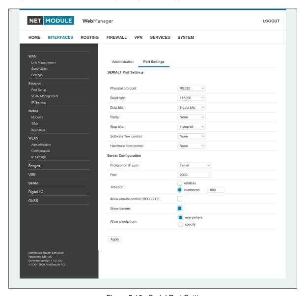
Figure 5.18.: Serial Port Settings
