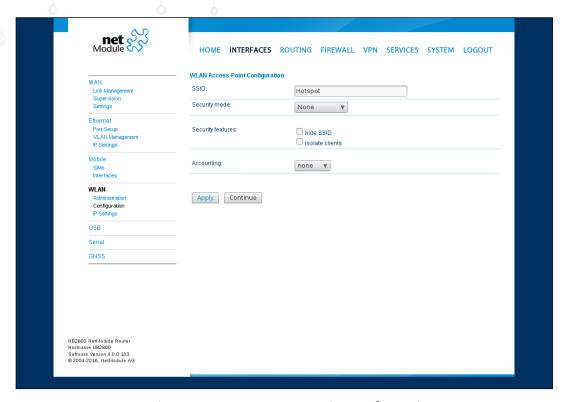
Figure 5.4: WLAN Access Point configuration
