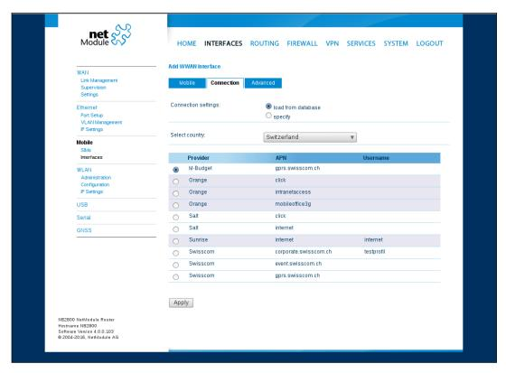
Figure 5.1: Mobile WWAN configuration
